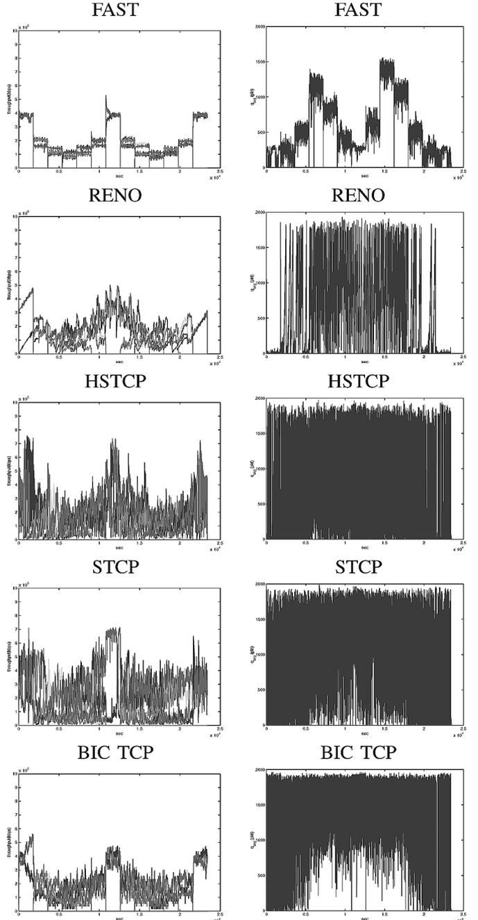
Fig. 5. Dynamic scenario II: throughput trajectory (left column) and Dumnyet queue trajectory (right column).
