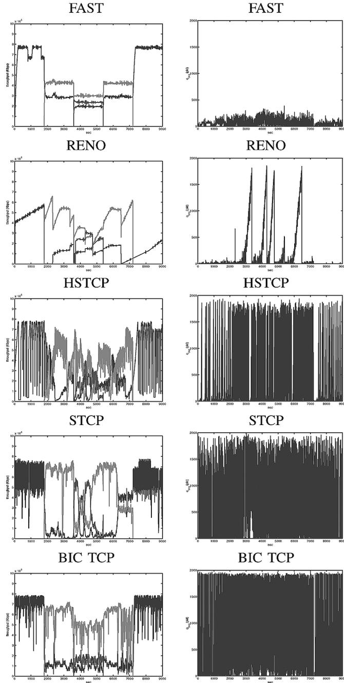
Fig. 3. Dynamic scenario I: throughput trajectory (left column) and Dummynet queue trajectory (right column).
