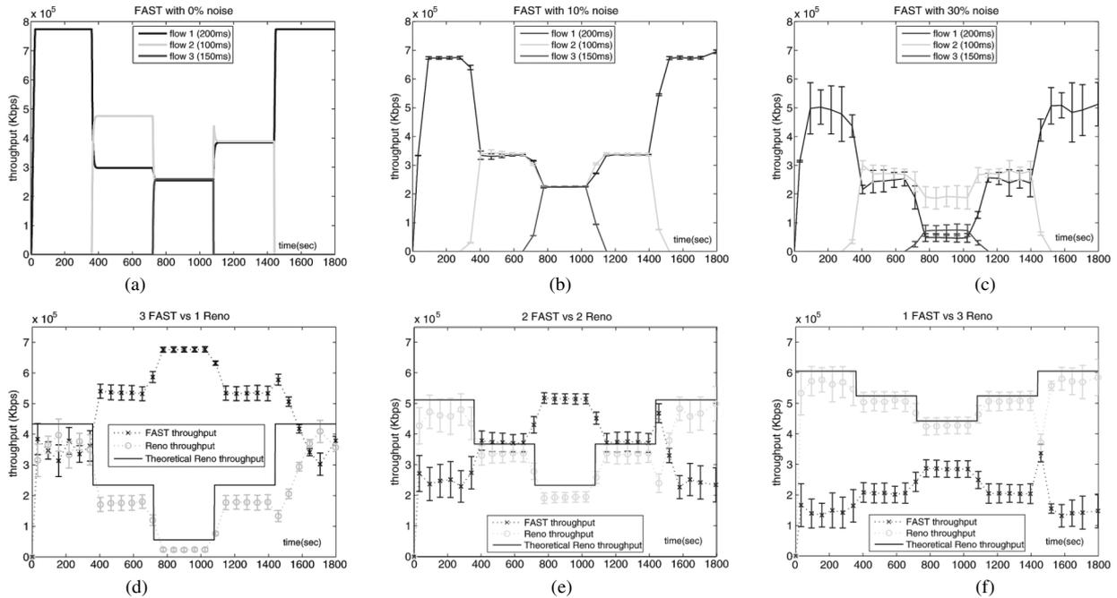
Fig. 7. (a) FAST with 0% mice traffic. (b) FAST with 10% mice traffic. (c) FAST with 30% mice traffic. (d) Three FAST flows versus one Reno flow. (e) Two FAST flows versus two Reno flows. (f) One FAST flow versus three Reno flows.
