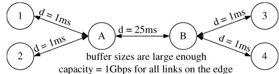
Fig. 8. Topology with multiple bottlenecks.
