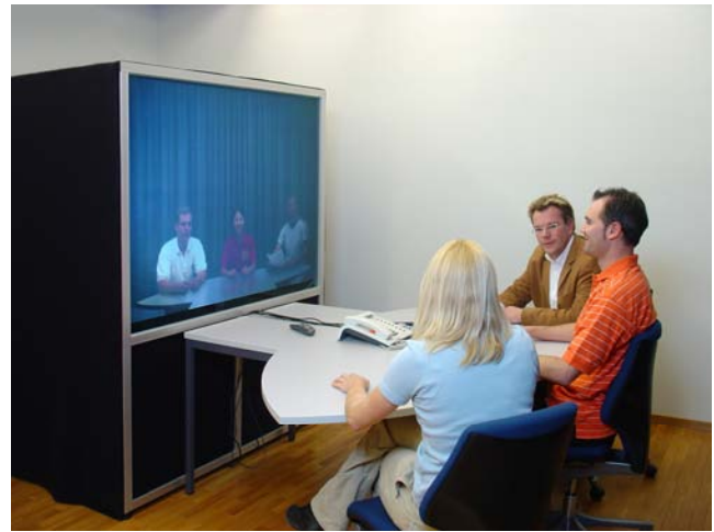
Figure 8: Networked group discussion using two HoloPorts, one for each group. The tables are both placed adjacent to the HoloPorts' screens to give the conferees the sensation of sitting virtually at the same conference table.
