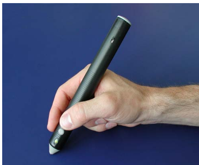
Figure 4: Infrared pen for on-screen interaction. The pen includes left and right mouse-click functionality. The devices' electronics was taken from a commercially available digitizer pointer.
