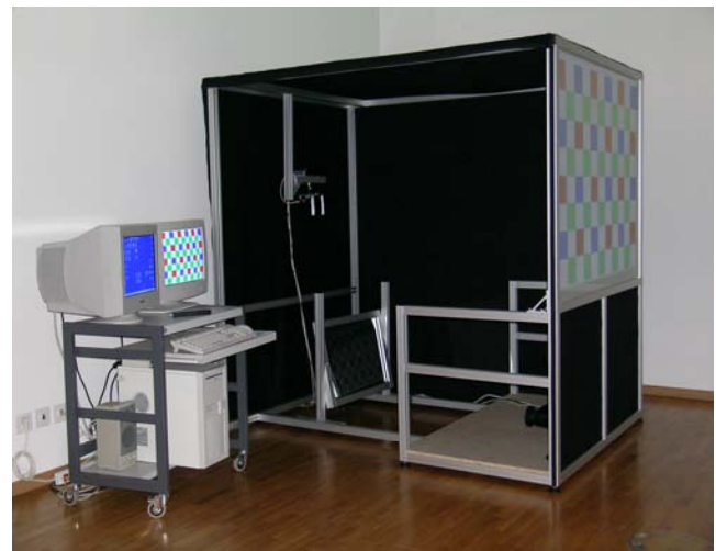
Figure 2: HoloPort prototype. For a better inside view, the light absorbing drapery is removed on one side.
