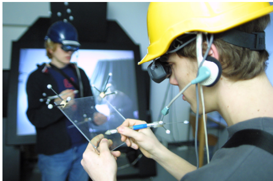
Figure 2: Immersive multi-user setup with two HMDs and large screen showing augmented camera view.
