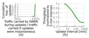
Figure 18: (a) SWAN carries close to optimal traffic even during updates. (b) Frequent updates lead to higher throughput.
